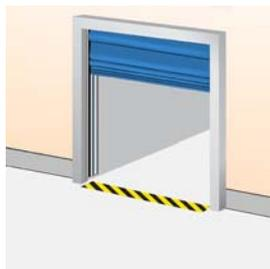
When it is unnecessary or undesirable to fully open a door, an absolute encoder is used to configure a reduced opening position.
