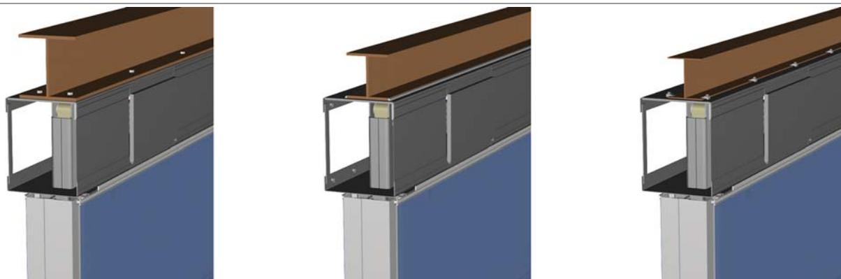
Fitting in door opening (header box screwed, welded or fixed beam clamps).
