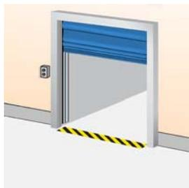
An extra control box is installed outside the building or inside close to the door if the main control unit needs to be installed away from the door opening. Installed on the inside or outside wall beside the door.
