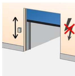
In case of main supply failure or emergency situations, it may be necessary to be able to open the door. The UPS battery stores enough power for one emergency opening cycle. Installed on the inside wall beside the door.
