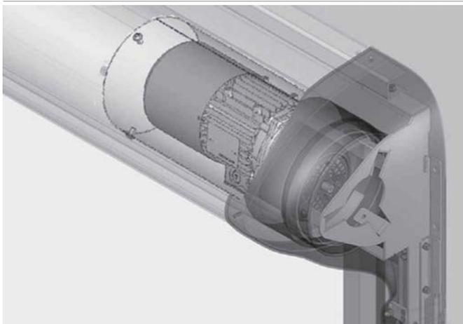
The operator is always placed on the right side of the door. Make sure the operator is accessible for service/maintenance.
