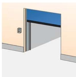
An extra control box is installed outside the building or inside close to the door if the main control unit needs to be installed away from the door opening. Usually combined with reduced opening. Installed on the inside or outside wall beside the door.
