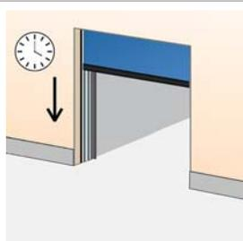
A programmable timer that closes the door after a specified time, counted from either the fully open position and/or from passing through the photocell beam. Usually also a switch on the control unit is used to turn to manual closing. Adjustable micro switches in control unit.
