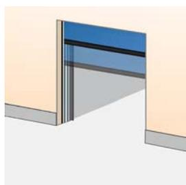
When people pass through the door, it may be unnecessary to fully open a door. A manual (pedestrian) command can trigger a reduced door opening, while a radar or magnetic loop still triggers a full door opening. Pre-fitted micro-switch to be activated in control unit.
