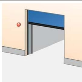
An orange warning light on each side gives information on the current door behaviour. Flashing light seconds before and during door movement. Installed on the inside and outside wall beside the door.
