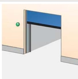
A green warning light installed on each side of the door indicating the open position of the door by continuous light signal.
