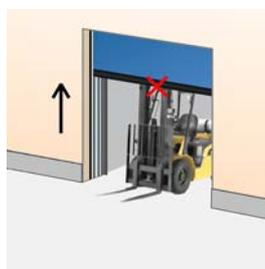
All doors are equipped with an edge activator. A wireless edge activator in the bottom seal detects any obstruction under a closing door and reverses the door. Installed in the bottom edge.
