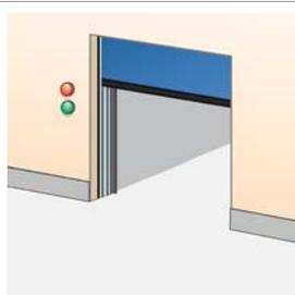
If traffic through a door needs to be directed; two red and two green traffic lights can be installed to indicate traffic direction. From the side where a vehicle is first detected to approach the door, the green traffic light comes on. The opposing side shows a red traffic light. Traffic from this direction must give way to the other. Usually installed in e.g. parking garages. Installed on the inside and outside wall beside the door.
