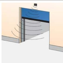
An infrared sensor above the door detects an object (person, vehicle) within a specified distance from the door and opens the door automatically. This is an ideal solution for frequent vehicle or personal traffic. Often combined with automatic closing. Installed on the inside or outside wall above the door.
