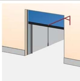
A pull-rope switch above the door opening can be operated from e.g. a forklift truck. Pulling the rope opens the door. Installed on the inside construction above the door.
