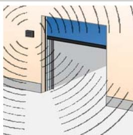
An acoustic signal is given, starting ...ms before the door begins to close and continues until the door is fully closed. Installed on the inside and outside wall beside the door.
