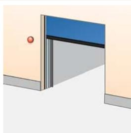
A red warning light on each side gives information on the current door behaviour. Flashing light seconds before and during door movement. Installed on the inside and outside wall beside the door.
