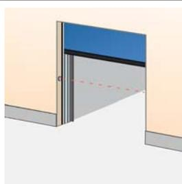
A set of a photocell transmitter and receiver is installed in the door opening. If the photocell beam is interrupted during closing, the door will stop in less than 30 mm and reverse to the fully open position. Installed in the door opening 300 mm from floor level.
