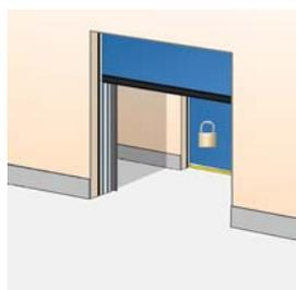
Developed for climate control or safety; If door A is open, door B cannot be opened. If door B is open, door A cannot be opened. An interlocked door can remember an up-command, if selected via a micro switch. Optionally an external locked switch can be installed to deactivate it.
