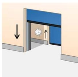
Developed for climate control or safety: Other than the interlock, door B will open automatically when door A is closed. Circuit card Installed in control unit. Optionally an external locked switch can be installed to deactivate it.
