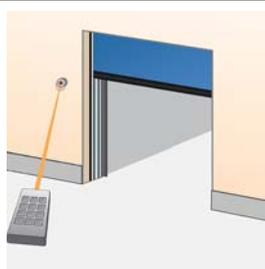
A hand-held radio transmitter allows door operation from a vehicle or any position within 50-100 meters from the receiver and aerial at the door. For closing, the door can be provided with a photocell beam. Receiver installed in control unit, antenna installed on the wall beside the door.
