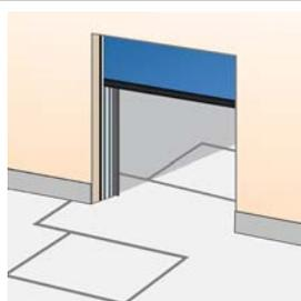
A sensor in the floor detects a metal object (usually forklift trucks, pallet trucks) and opens the door automatically. This is an ideal solution for frequent vehicle traffic. Installed on the outside, inside or both sides of the door in the floor.
