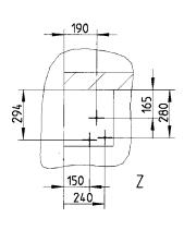
Inspect the install location concerning the required anchoring points and set-up conditions. It may be necessary to prepare a support construction or other suitable anchoring possibilities. The head plates should be bolted to a steel support construction or to a concrete element.
