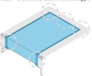
The frame is the leveller's connection point to the building. The replacement Pit-frame system requires that the concrete pit and the old existing steel profile in the concrete are strong enough to cover the loads of a new leveller. The Pit-frame is designed to designed to take out the old leveller completely. If these requirements are not fulfilled, then the solution is a
