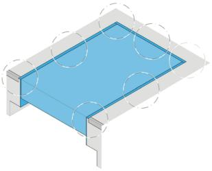
The frame is the leveller's connection point to the building and a rigid support for the leveller. The replacement F-frame system requires that the concrete pit and the old existing frame are strong enough to cover the loads of a new leveller. The F-frame is designed to weld the leveller directly to the existing leveller's frame.
