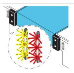
Crawford Dock-IN White & Red is the optimum combination of both systems for easy and safe docking. The white LEDs provide the visual target and the red LED positions the truck at the right distance to the dock. The white guiding LEDs turn off when the truck is detected and at the same time the red LED turns ON. Crawford Dock-IN White & Red guide the truck driver in the best possible way for an easy and safe docking.
