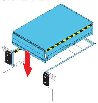
Install the new leveller according to the the basic principles of a Pit model; weld the rear frame to the existing steel profile in the concrete, the front part of the leveller is supported directly by the floor of the closed pit or by strong steel brackets of the open pit.
