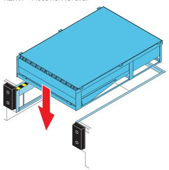
Weld the replacement leveller directly to the old existing leveller's frame on all three sides.
