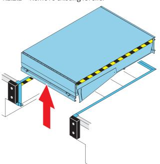
Remove the complete steel structure.
