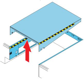
Remove the old leveller. Leave the old leveller's steel frame in the pit.
