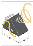
The wheel chock has a sensor to detect the presence and position of the vehicle and is connected to the dock leveller control panel. If no vehicle is detected, the docking station is blocked for safety reasons. Furthermore, the wheel chock prevents the vehicle from moving during loading/unloading.
