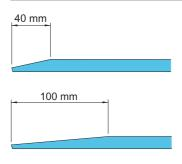
The standard steel lip is 40 mm bevelled.
