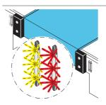
ASSA ABLOY Dock-IN White & Red is the optimum combination of both systems for easy and safe docking. The white LEDs provide the visual target and the red LED positions the truck at the right distance to the dock. The white guiding LEDs turn off when the truck is detected and at the same time the red LED turns ON. When the truck is leaving the white LEDs turn ON. ASSA ABLOY Dock-IN White & Red guide the truck driver in the best possible way for an easy and safe docking.
